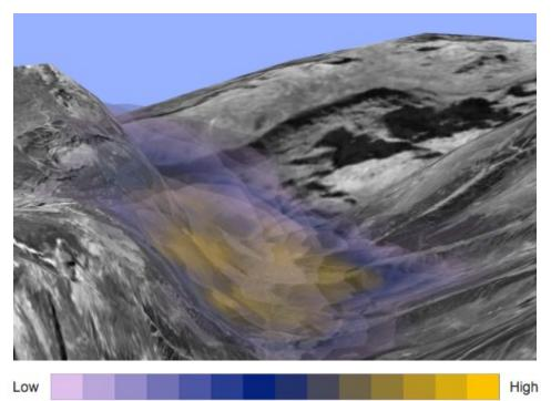
This sophisticated simulation of atmospheric  $CO_2$  concentration has high spatial and temporal resolution, is based on the laws of conservation of momentum, energy and matter, and is itself nested inside a simulation that spans a large portion of Europe.
