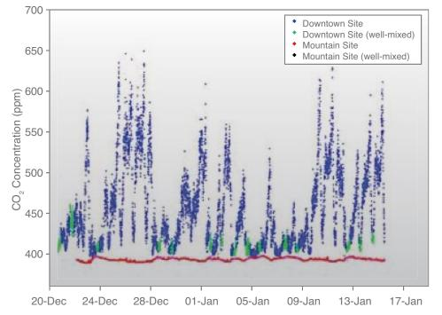
**Mountain measurements (red)** are flat because air from the city does not usually travel up to the station, so this measurement gives a baseline of how much CO<sub>2</sub> is present in the air coming into Davos
